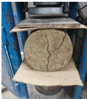
Figure 6. Diametral compression tensile strength test on cylindrical samples.
