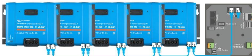
With VE.Can up to 25 Charge Controllers can be daisy-chained and connected to a Color Control GX or other GX device Each Controller can be monitored individually, for example on a Color Control GX and on the VRM website
