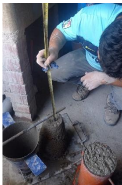
Anexo 6.3: Slump 2" – Concreto Experimental 0.05%NG + 5% RL
