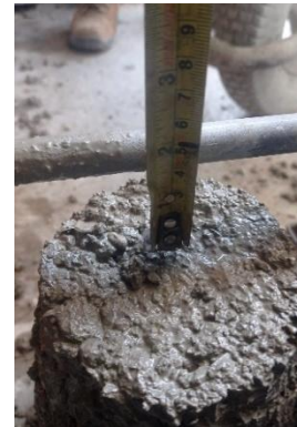
Anexo 6.4: Slump 2" – Concreto Experimental 0.1%NG + 5% RL
