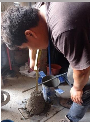
Anexo 6.4: Slump 2.5" – Concreto Experimental 0.05%NG + 3% RL
