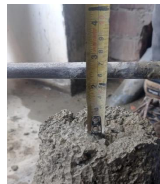
Anexo 6.4: Slump 2.5" – Concreto Experimental 0.1%NG + 3% RL
