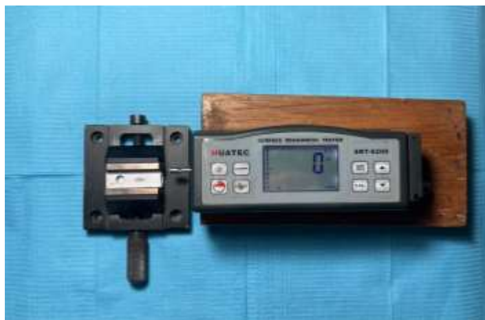
Figura 5: Rugosímetro (HUATEC Industry Instrumentation, modelo SRT-6200).
