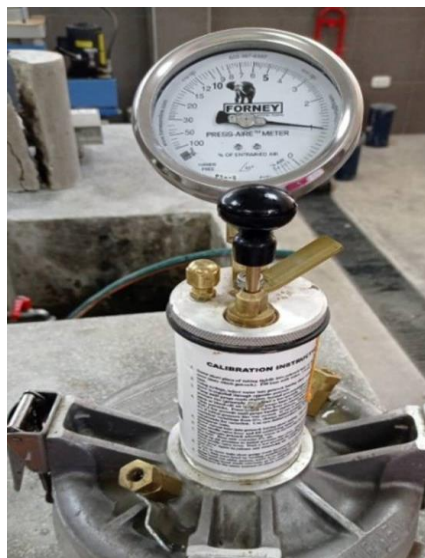
Fig.3 - Air Content Test
