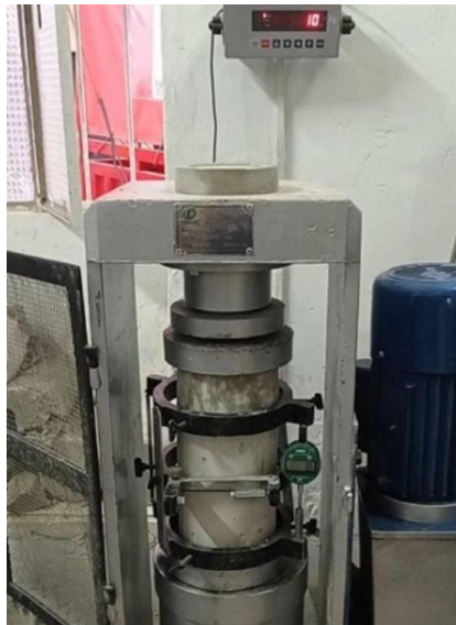
Fig.5 - Modulus of Elasticity Test
