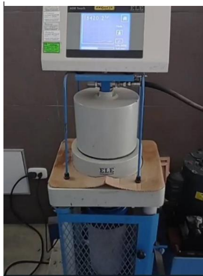
Fig. 4 - Compressive Strength Test
