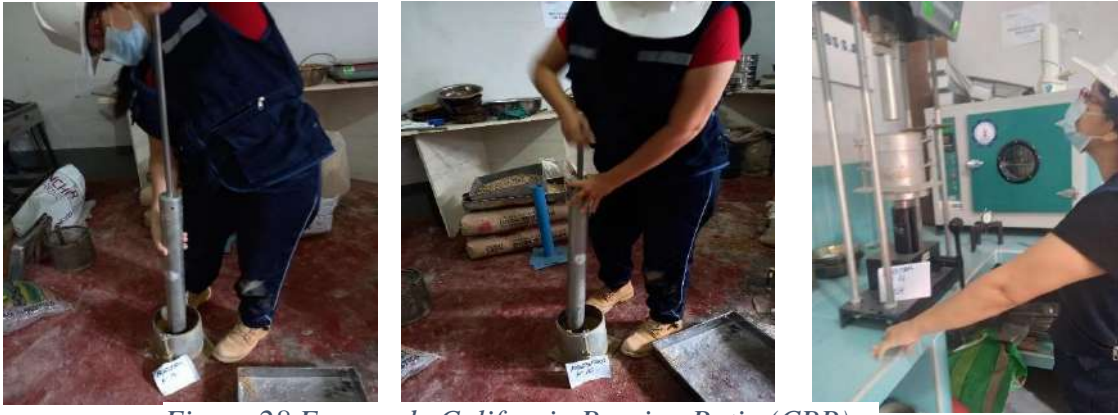
Figura 28 Ensayo de California Bearing Ratio (CBR)
