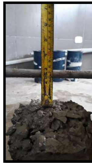
Anexo 16.6: Slump 2.75''- Concreto 10% V y 20% RCD
