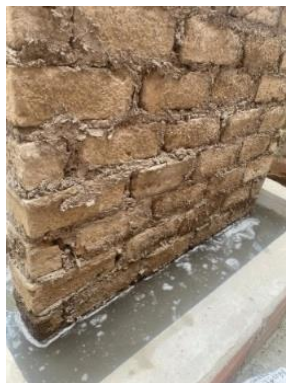
Figure 6. Samples for simulated flood testing of low walls
