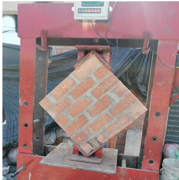
Figure 6: Axial compression test of walls.
