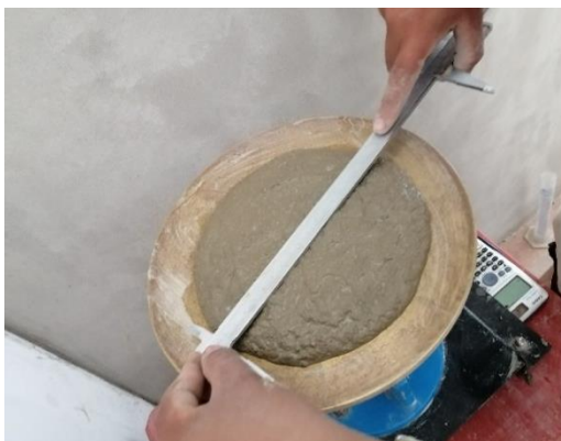
Figure 2: Measurement of mortar expansion.
