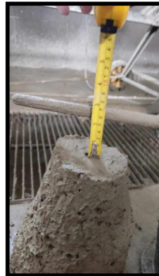
Anexo 12.4: Slump 2.5" – 20% Arcilla Expandida
