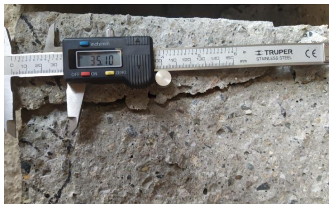
Figura N° 108: P01d - f'c 280 - a/c 0.53 - 100%AR - 0.05%NG.
